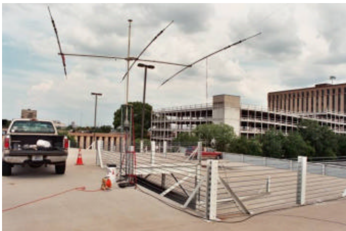
Extra 20/17/15M beam on a temporary mast and rotor strapped to the parking garage. This beam really helped the CW station.
